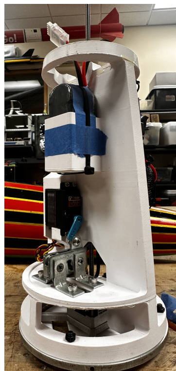
Figure 3.8: No damage was observed on GrAVE after launch.
