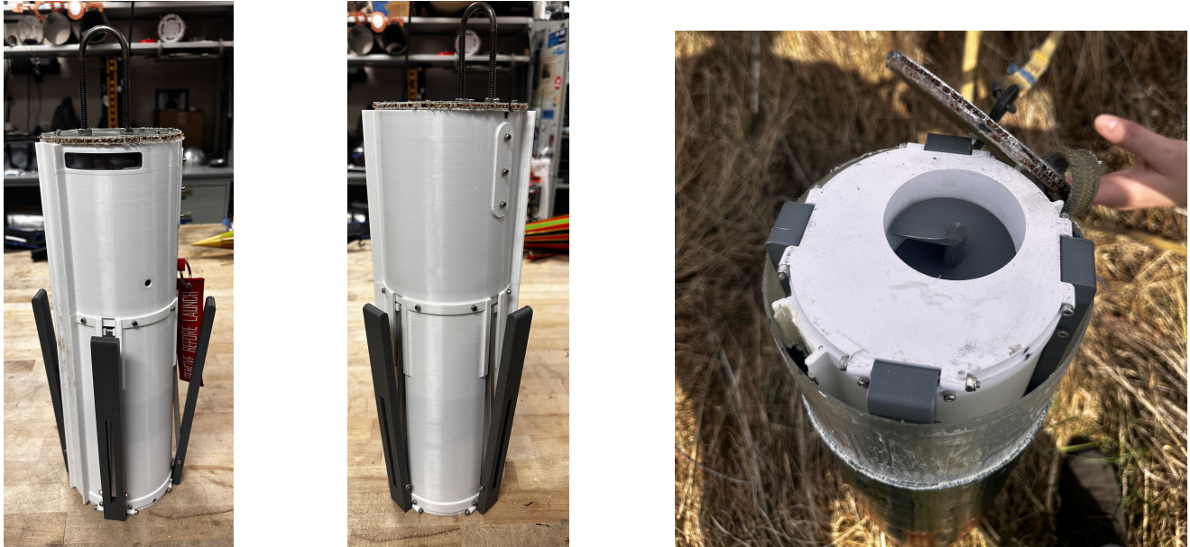
Figure 3.9: No damage was observed on ZOMBIE after launch.
