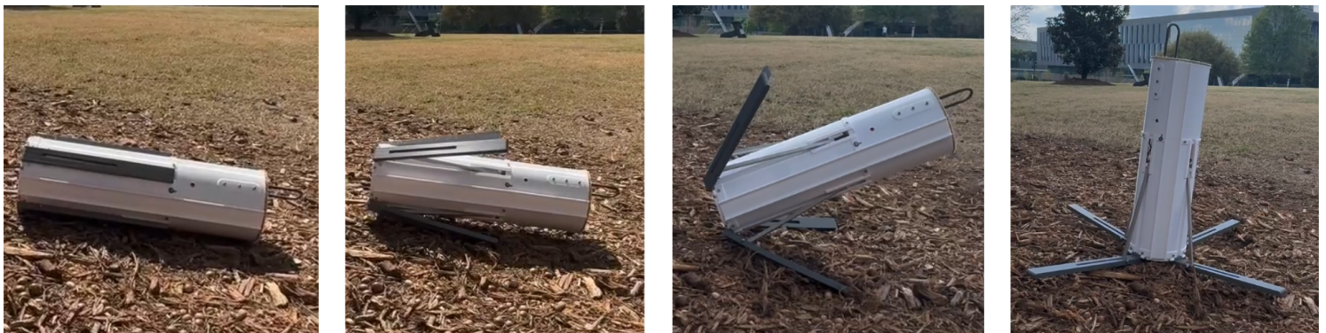
Figure 5.3: Results of the ZOMBIE Self-Righting test.
