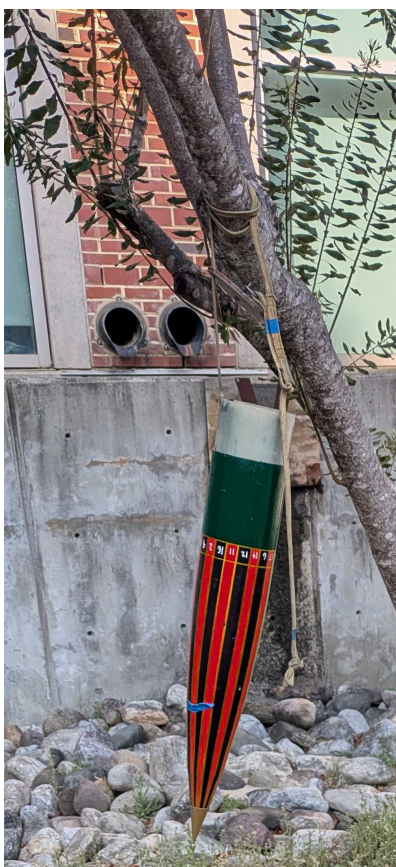
Figure 3.7: The payload hung from a tree to test ejection safety.
