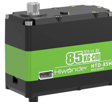
Figure 5.9: Hiwonder HTD-85H Servo and Encoder
