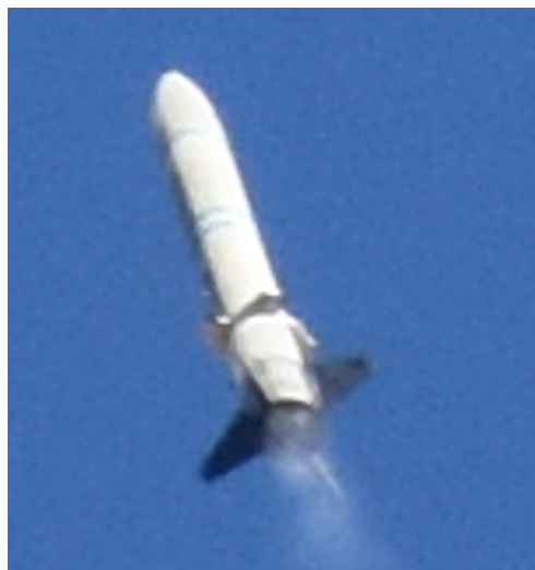
Figure 3.37: Air Brakes deployment during ascent.
