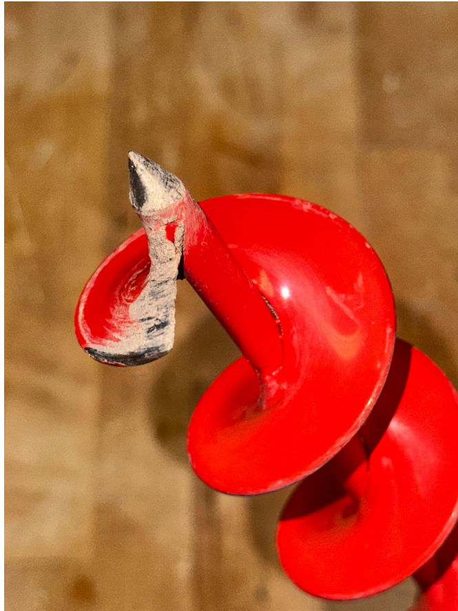
Figure 4.17: Sharpened tip of carbon steel auger.
