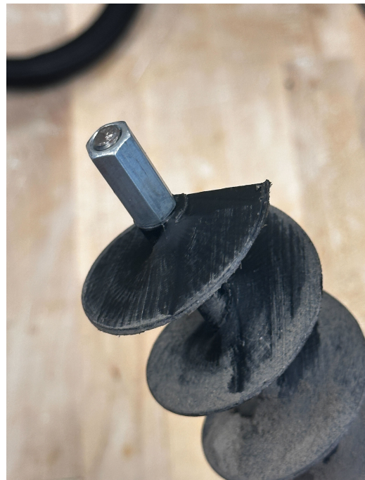
Figure 4.21: Threaded rod interface at top of auger.
