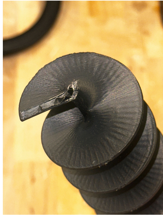
Figure 4.19: Failure point on PETG auger.
