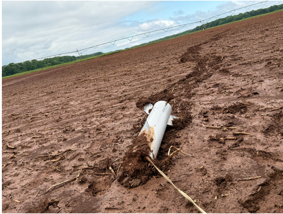
Figure 2.8: Fin Can after it was dragged by the wind
