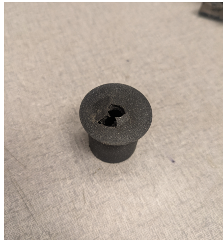
Figure 2.13: Bottom view of damaged 3D printed charge well.
