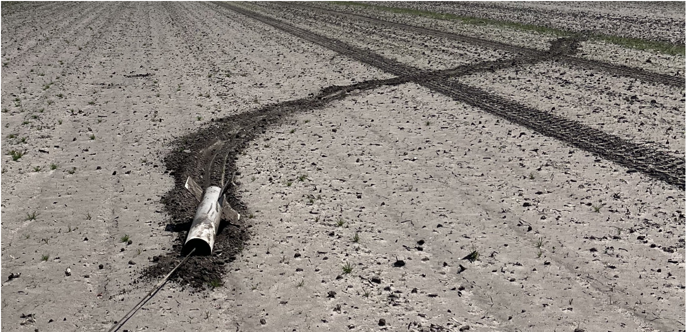
Figure 2.4: Fin Can after it was dragged by the wind
