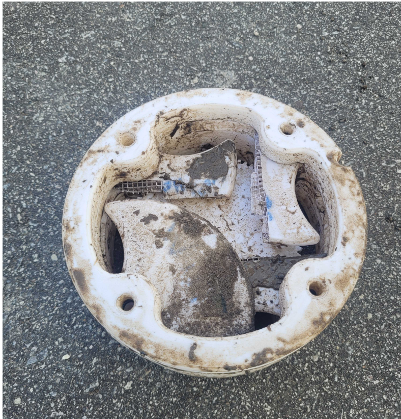
Figure 2.16: Damage sustained to the Air Brakes housing and fins.
