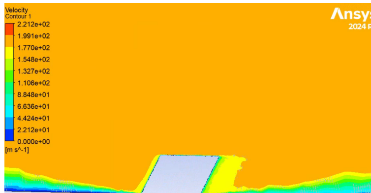
Figure 3.15: Final Fin Design Velocity Profile (600 fps)
