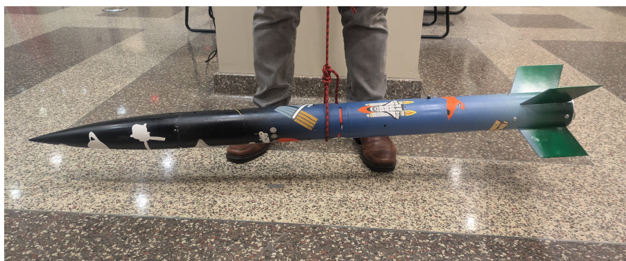
Figure 3.28: Balance point test to verify burnout CG position for the Subscale Launch Vehicle.
