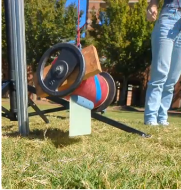
Figure 3.3: Example of fin system ground impact testing.
