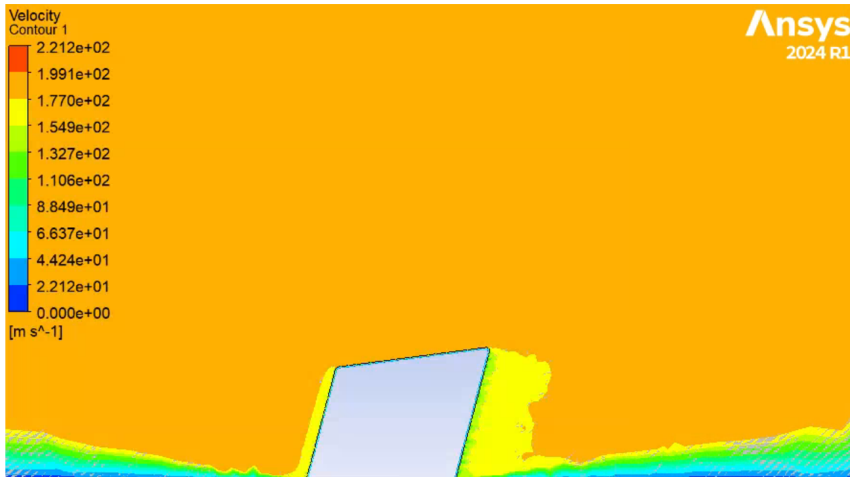
Figure 3.6: Velocity Profile of Swept Fin with Slanted Tip Chord at 600 fps
