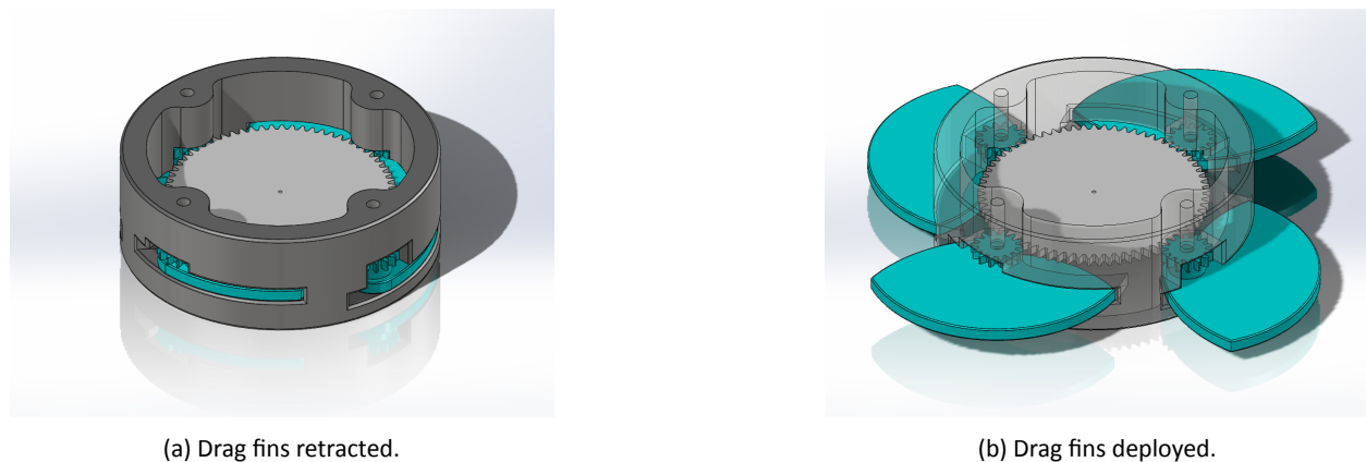
Figure 4.3: Air brakes deployment mechanism.
