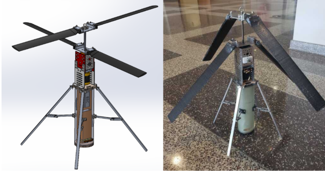
Figure 3.1: Final SAIL CAD and as-built configuration.
