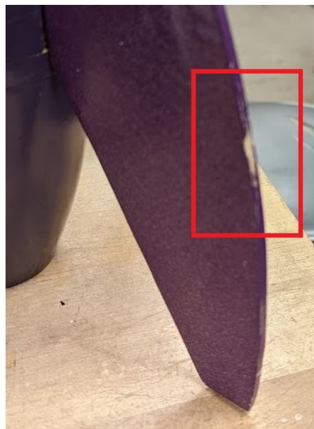
Figure 38: Damage on the leading edge of the fin sustained during landing.
