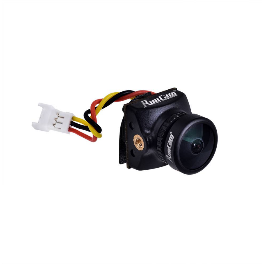
Figure 71: A commercially available FPV camera, the RunCam Nano 2. [20]
