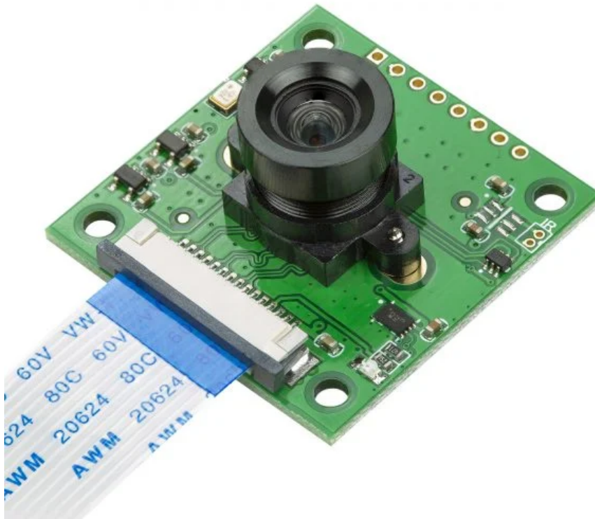
Figure 72: A commercially-available Raspberry Pi camera, the Arducam IMX219. [8]
