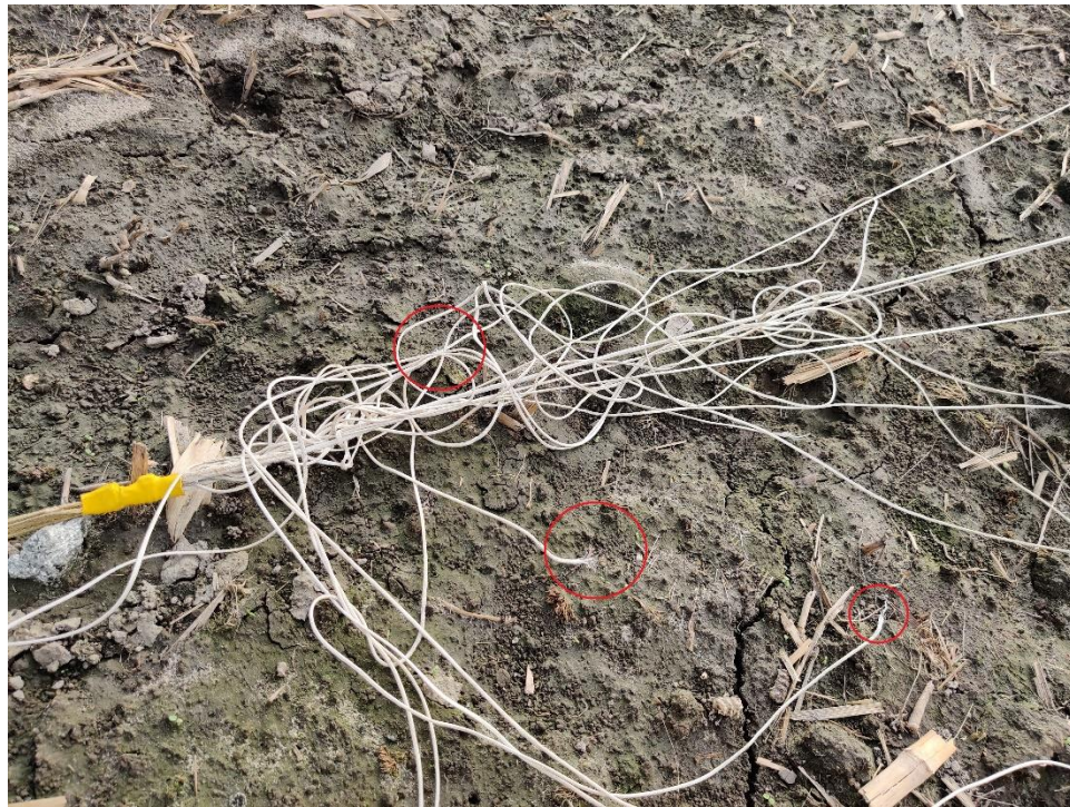
Figure 3-5 Severed Main Parachute Shroud Lines
