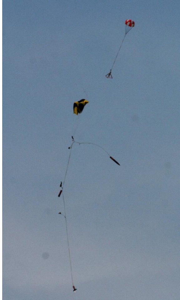
Figure 2-2 LOPSIDED-POS Descending Separately from Launch Vehicle
