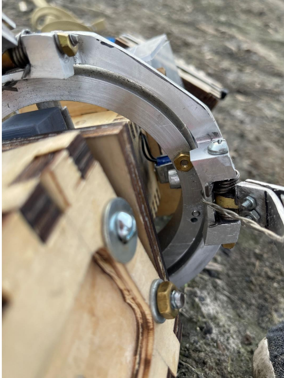
Figure 2-9 Loose Solenoid Bracket Bolt and Nut
