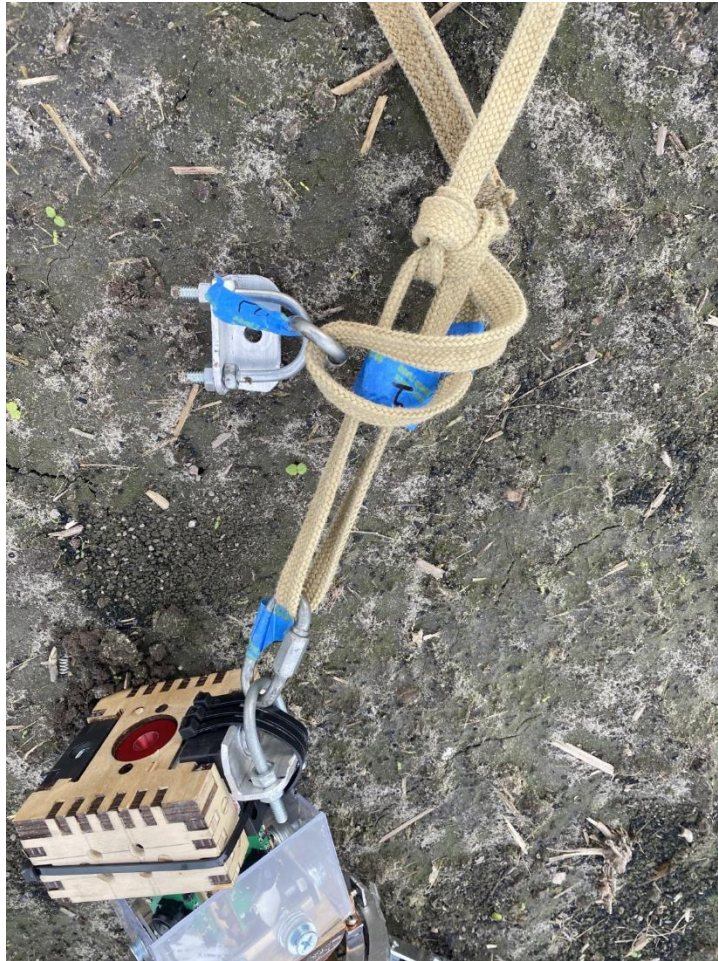
Figure 2-5 Electromechanical Locks, U-Bolt with Pins, and Payload Shock Cord
