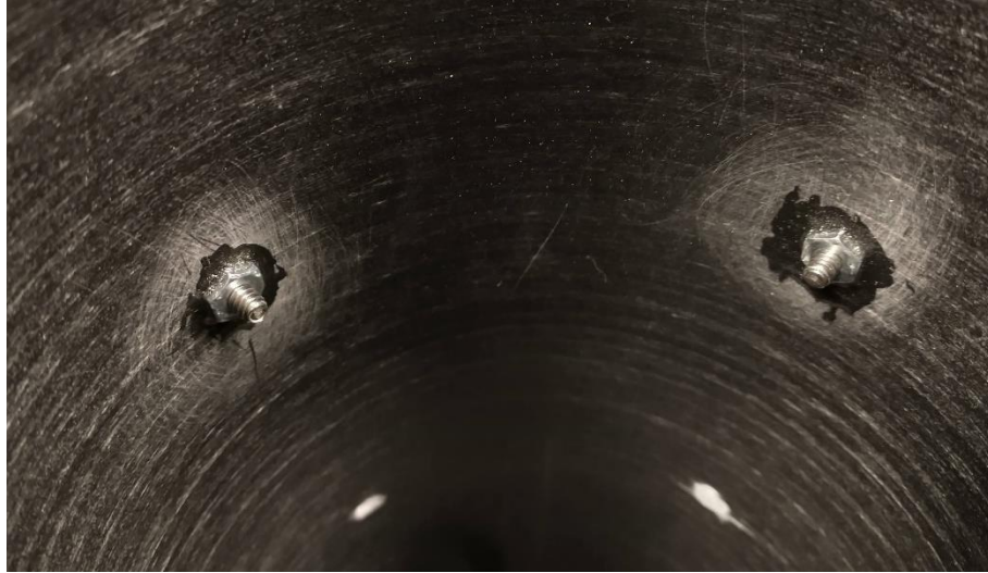
Figure 3-31 Nuts Secured to the Inside of the AV Bay
