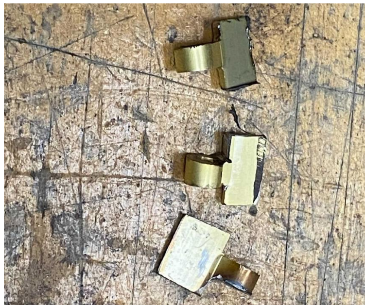
Figure 4-25 Leg Hinges Cut from Door Hinges
