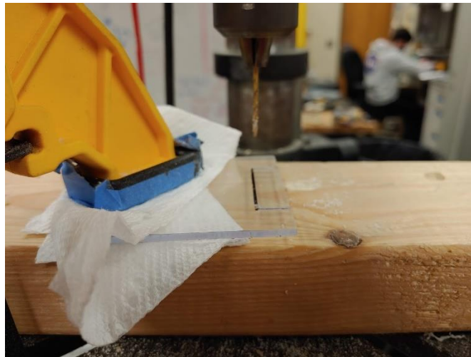
Figure 4-28 Perforating Polycarbonate with Drill Press
