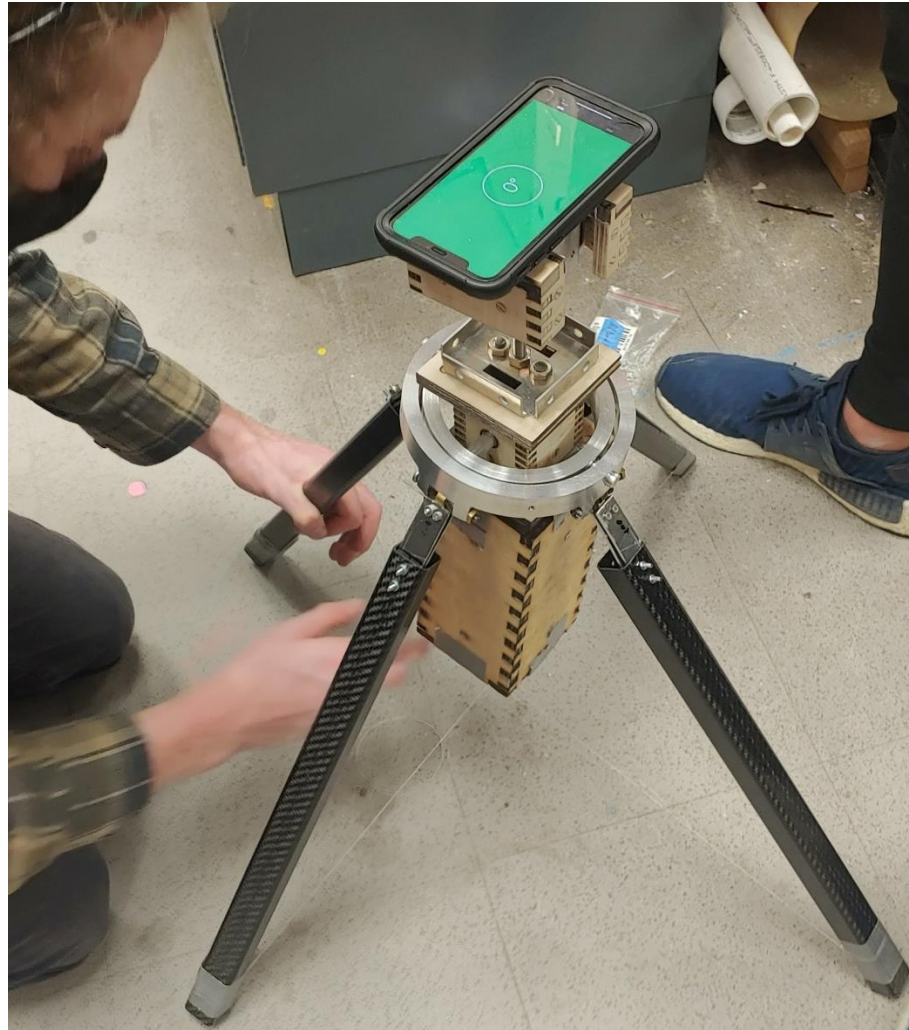
Figure 4-8 Level LOPSIDED Demonstrating Centered CG
