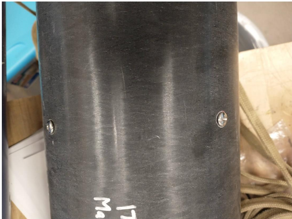
Figure 3-32 Bolted Connection between Main Parachute Bay and AV Bay
