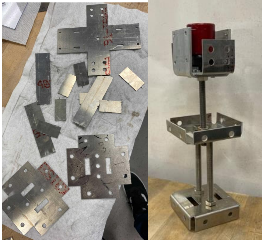
Figure 4-21 Metal Frame Unassembled (Left, with Other Metal Parts), and Assembled (right)
