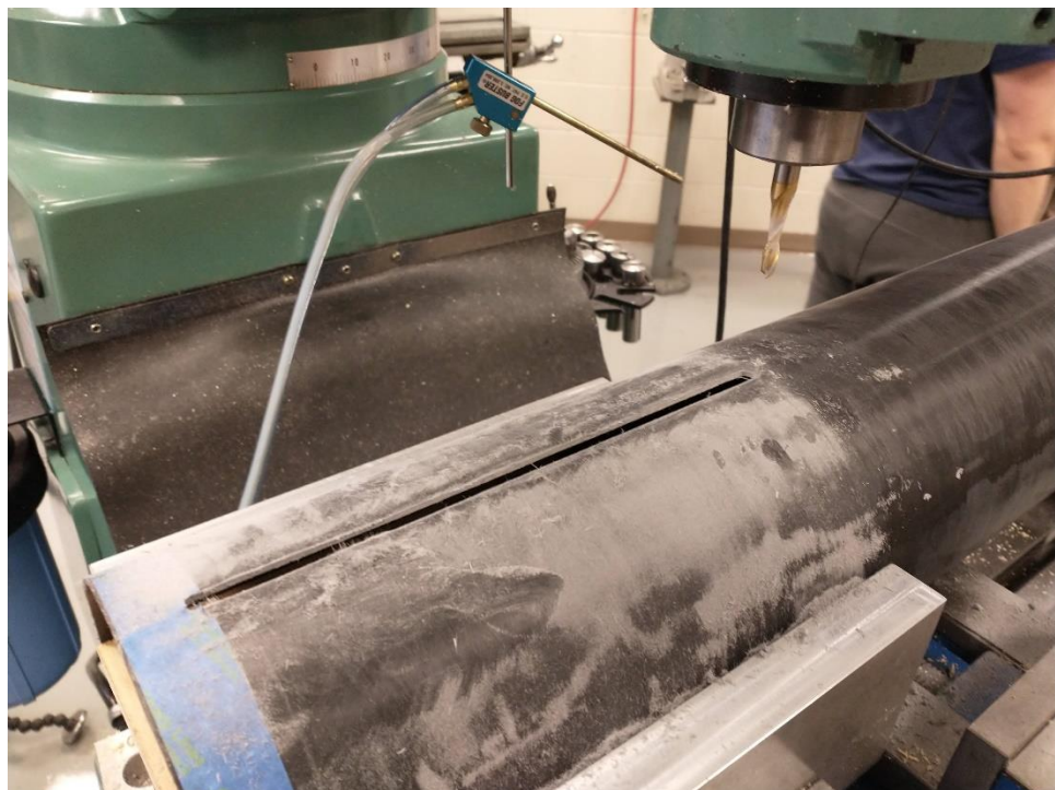
Figure 3-29 Fin Slots Cut by Mill
