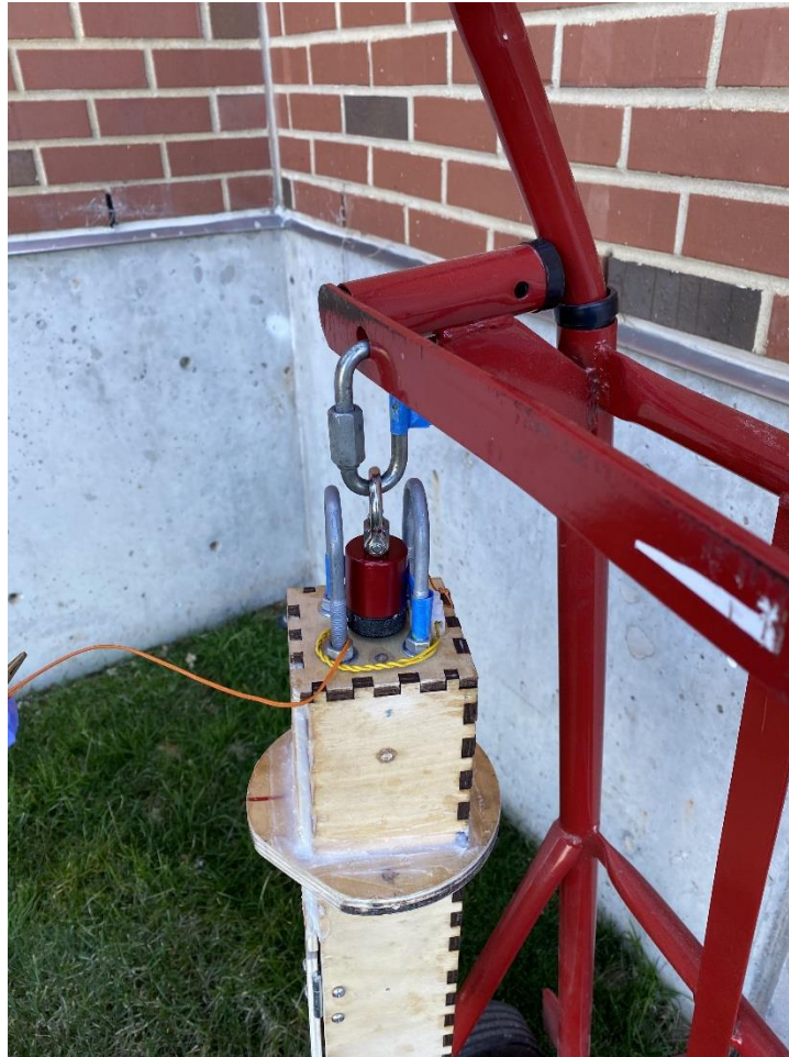
Figure 7-8 Mass Simulator Held on Test Rig by ARRD
