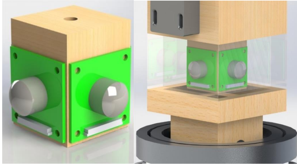
Figure 4-20 POS Camera Module and Mounting Fixture Located Within LOPSIDED Upper Section
