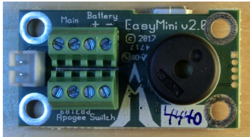
Figure 3-19 Altus Metrum EasyMini Altimeter
