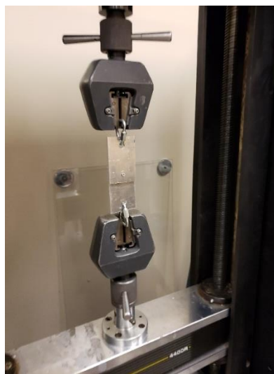
Figure 7-5 Fastener Loading Test Set Up
