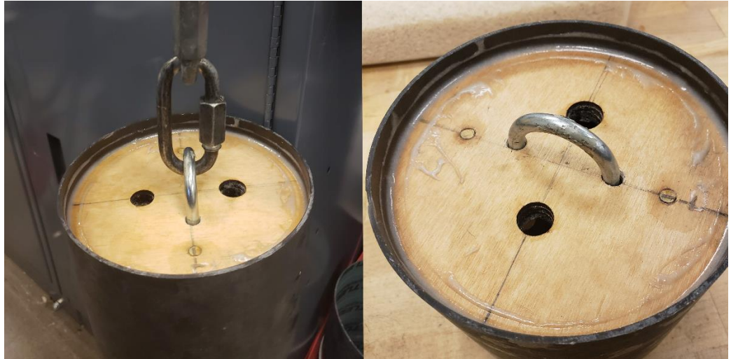
Figure 7-2 Epoxied Bulkhead – Before and After Testing
