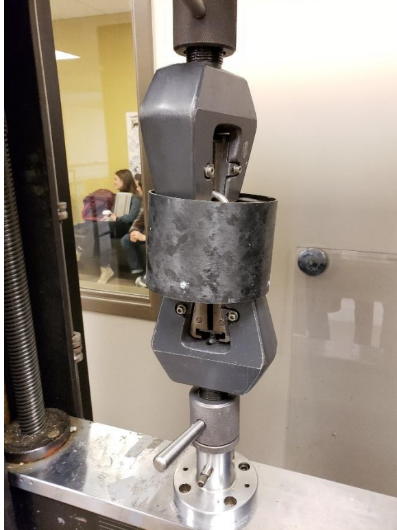
Figure 7-1 Bulkhead Tensile Loading Test Set up
