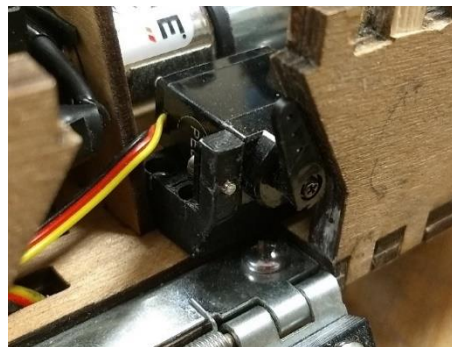
Figure 4-25 Caster Wheel Deployment Assembly
