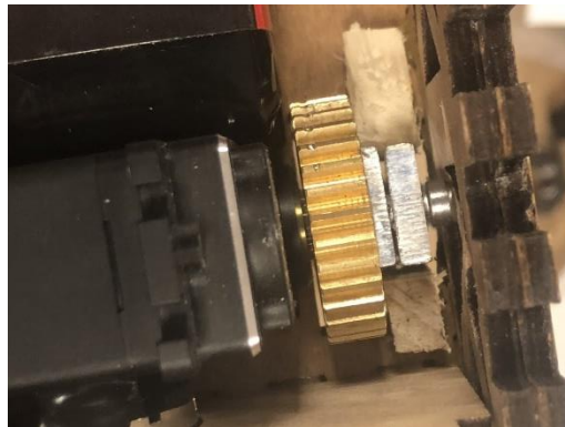
Figure 4-22 Shaped Wood to Hold Gear Bracket in Place
