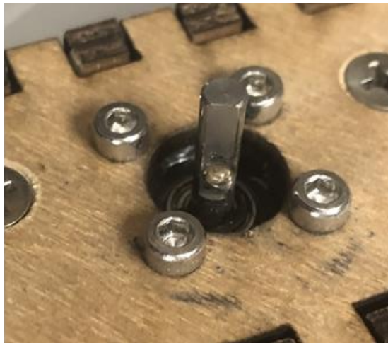
Figure 4-23 DC Motor Mounted to Chassis
