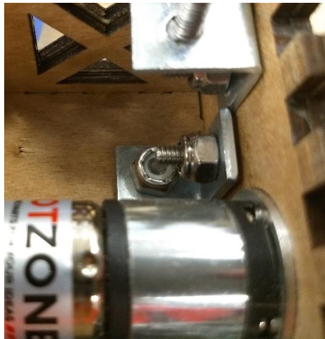
Figure 4-20 An L-bracket securing the BURRITO Plates
