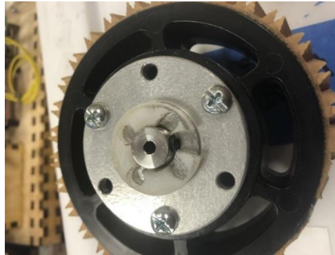
Figure 4-24 Wheel Assembly with Nylon Washer
