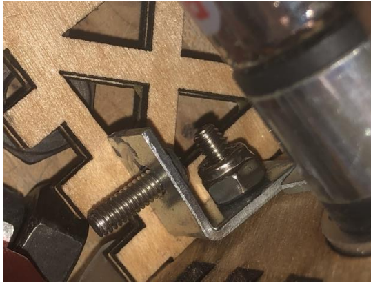
Figure 4-21 L-Bracket with adhered bolt
