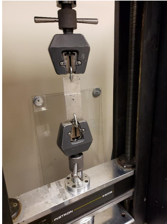
Figure 7-4 Shear Pin Test Set Up
