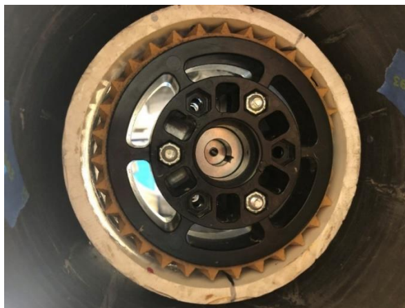
Figure 4-51 Aft Rover wheel in centering ring
