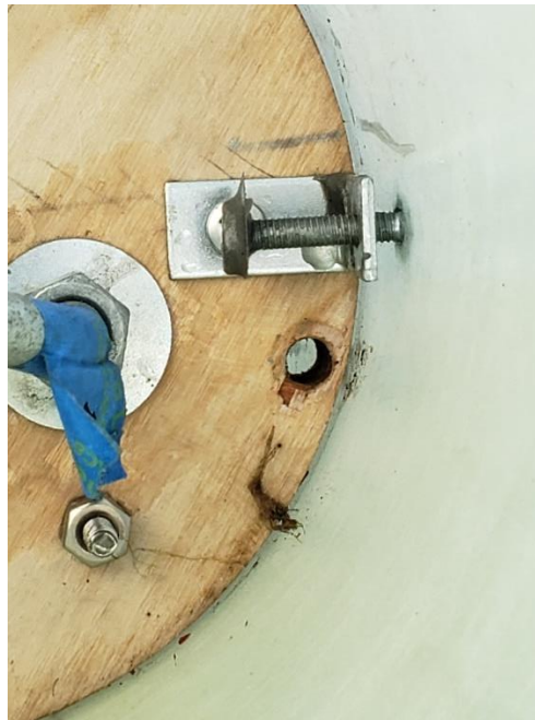
Figure 3-22 Nut Detachment in Nose Cone
