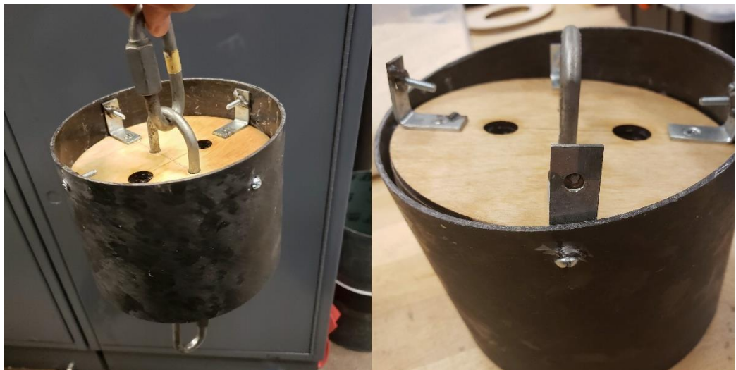
Figure 7-3 Bolted Bulkhead – Before and After Testing
