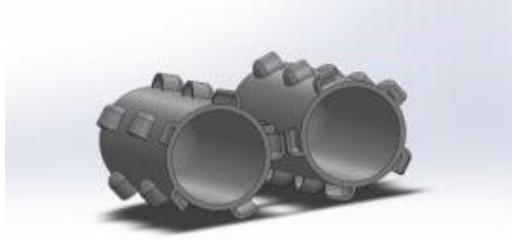
Figure 4-3 Rotating Drum design, section view
