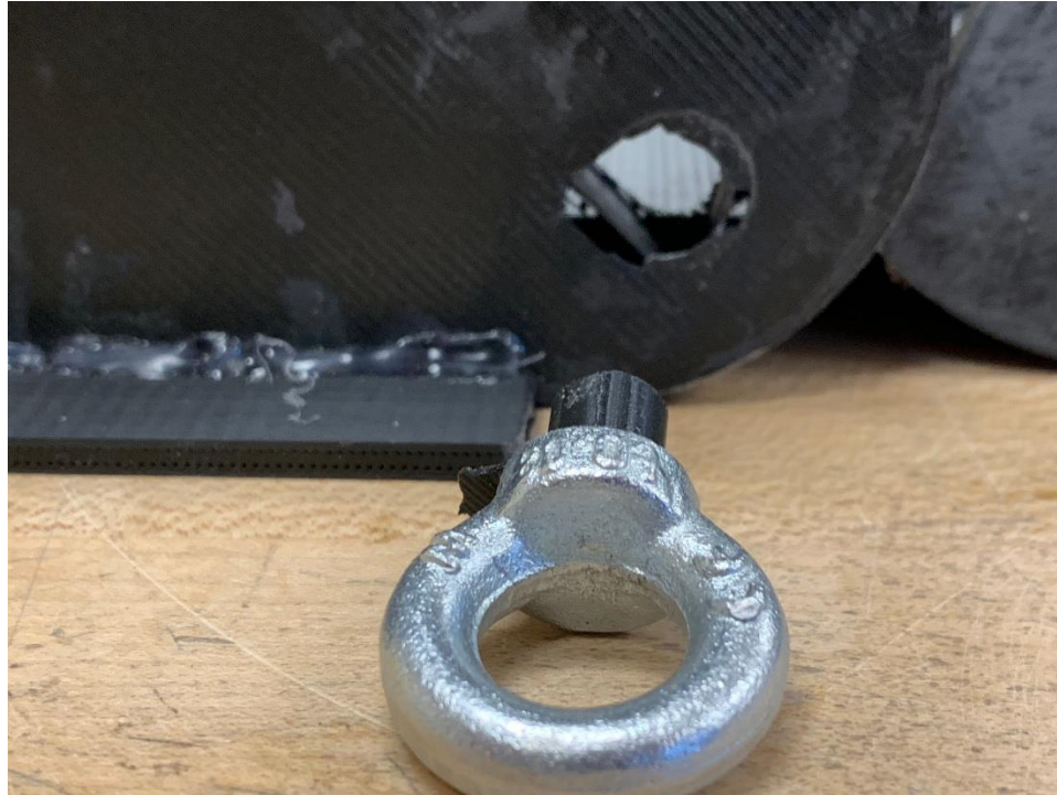
Figure 2-1 Damage to Payload Retention System
