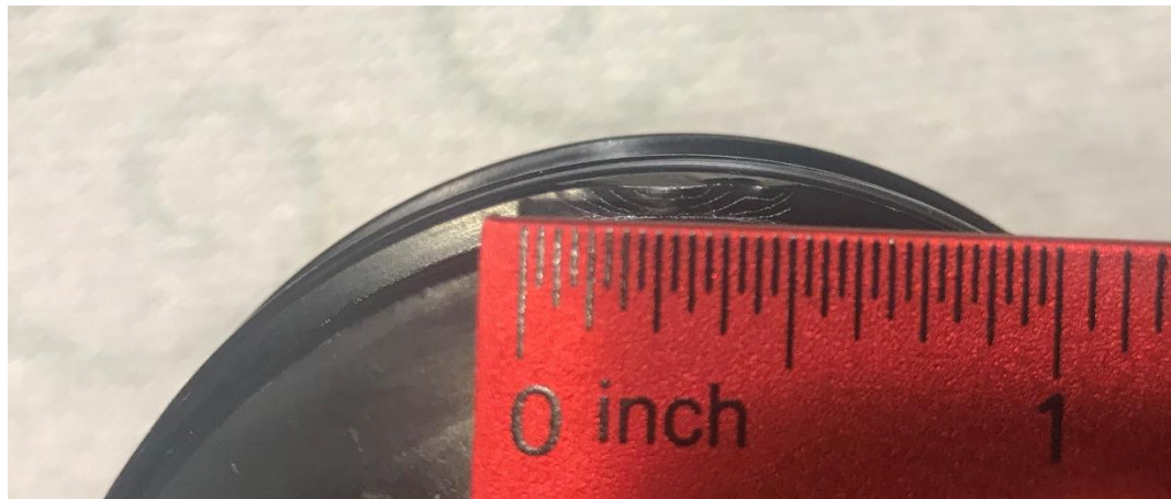
Figure 3-4 Damage to Motor Casing Forward Closure
