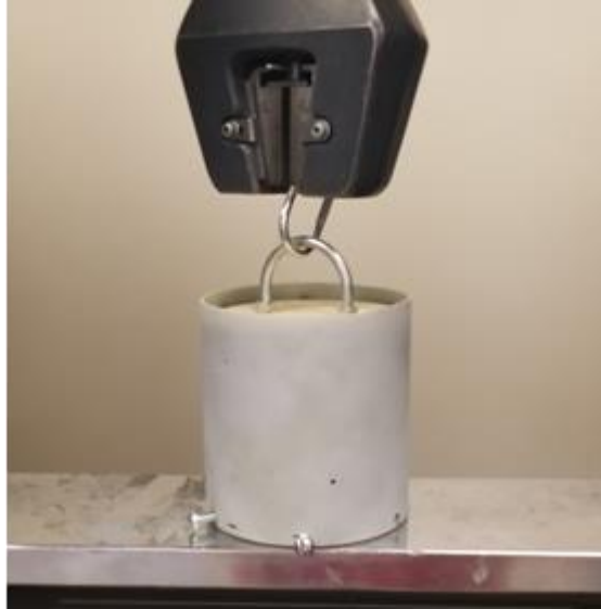
Figure 6-1 Bulkhead Failure Testing Setup – Run 1
