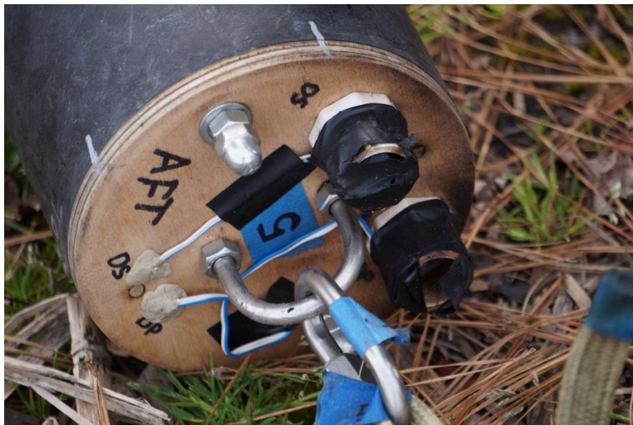
Figure 10-14 Drogue parachute deployment charges after deployment
