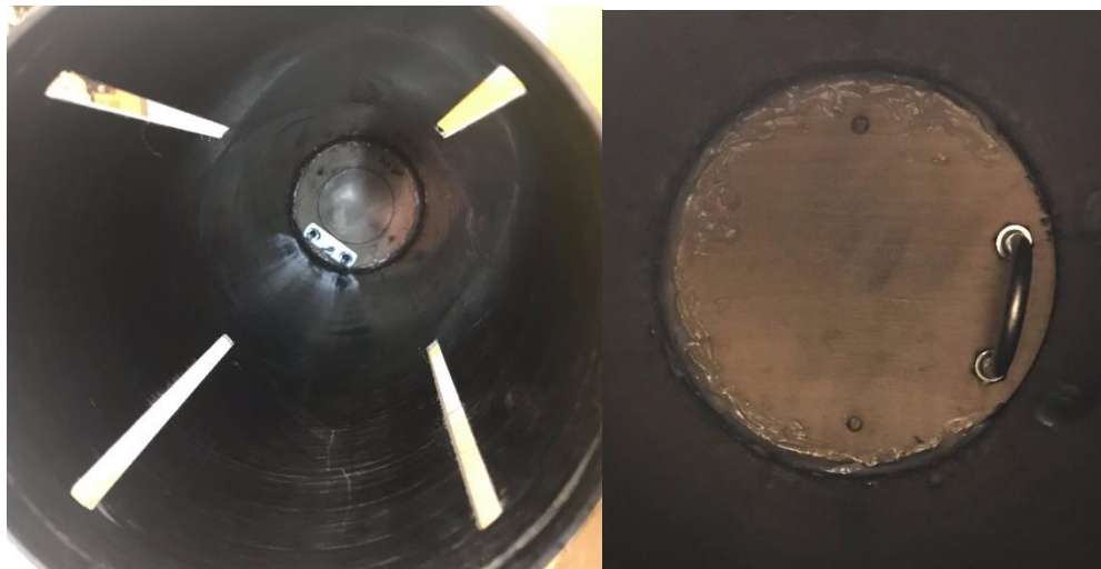
Figure 3-19 Fin Can Bulkhead Epoxy Fillet
