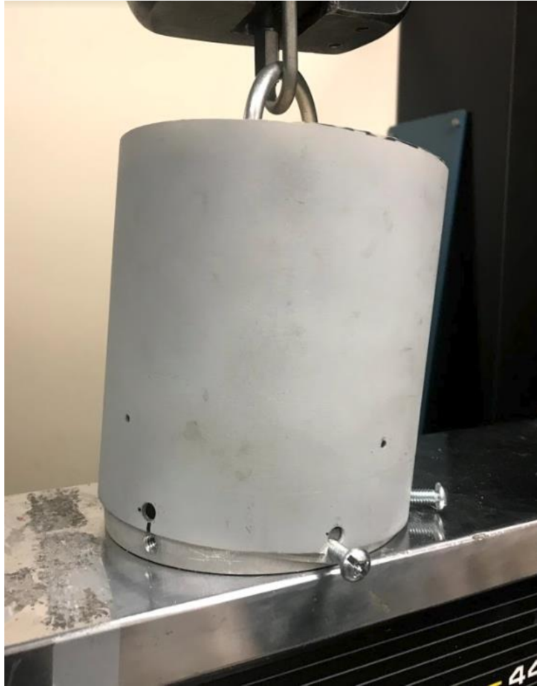
Figure 6-4 Bulkhead Failure Test Setup and Fiberglass Failure
