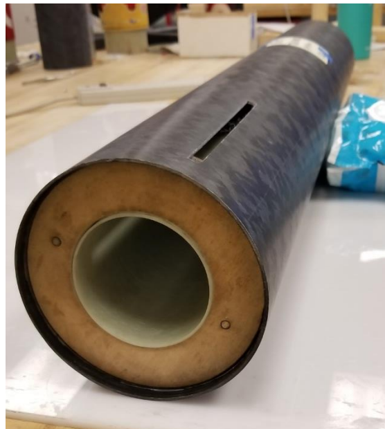
Figure 3-17 Fin Can Bulkhead Alignment
