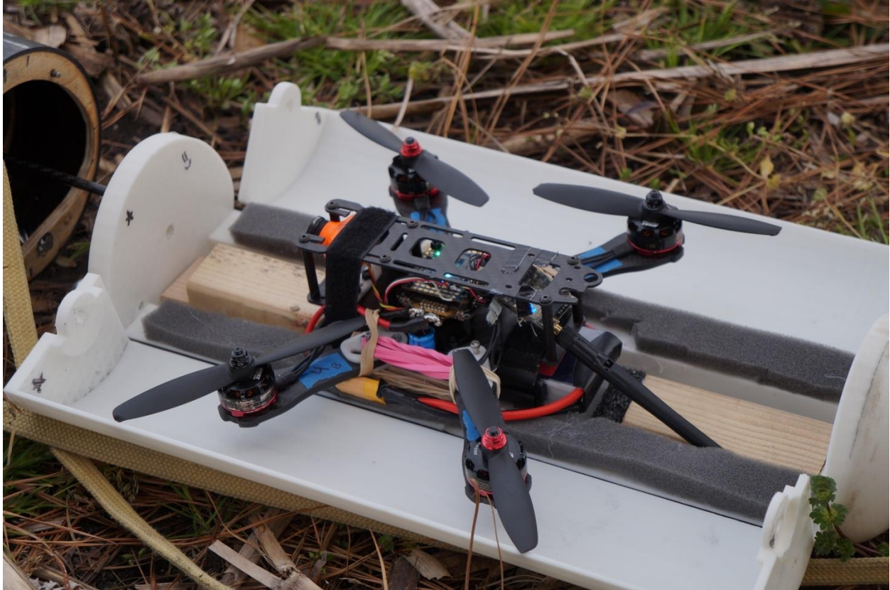
Figure 10-13 UAV emerging from the pod with damaged antennae
