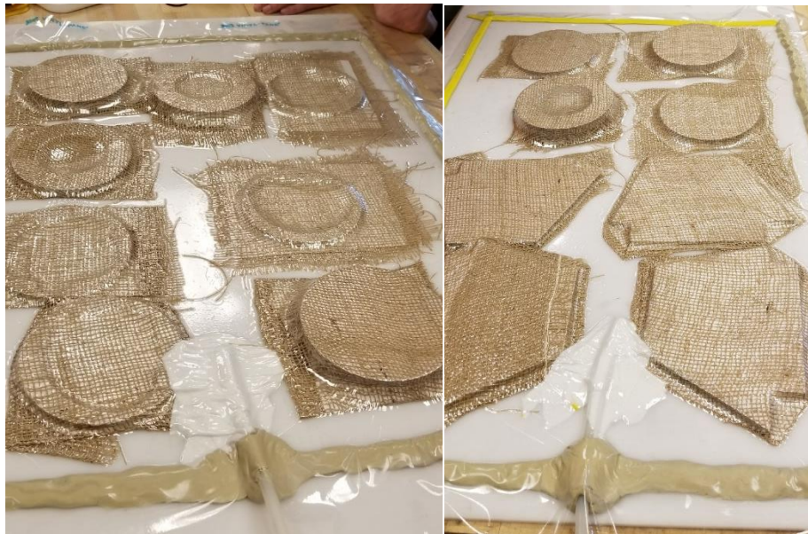
Figure 3-15 Bulkheads and Fins Under Vacuum
