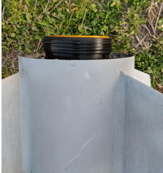
Figure 10-3 motor installation profile view prior to motor retainer attachment
