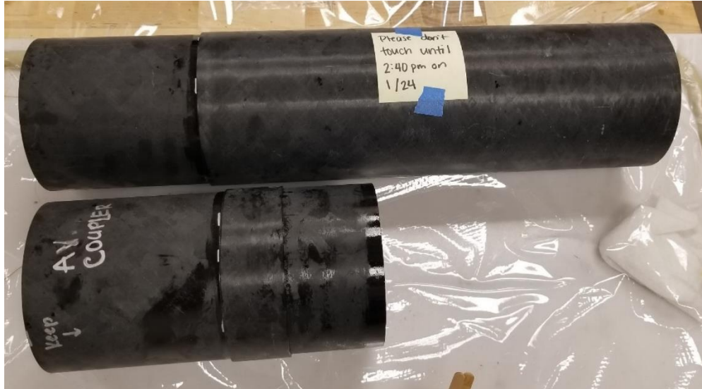
Figure 3-9 Payload Bay and AV Bay Coupler Attachments
