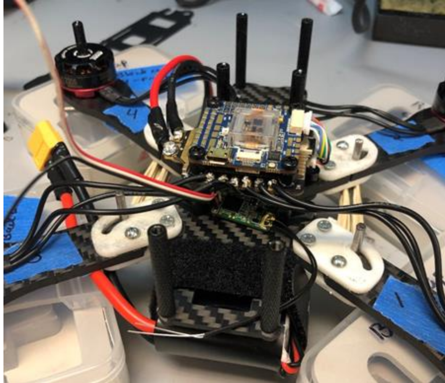
Figure 5-8 UAV Motors Wired to Flight Controller
