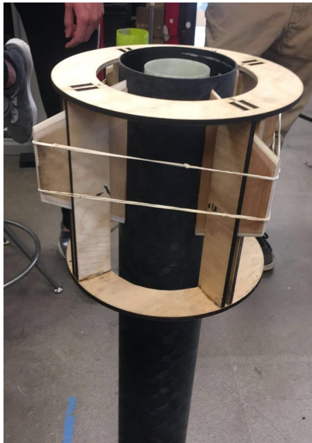
Figure 3-20 Fin Support While Curing
