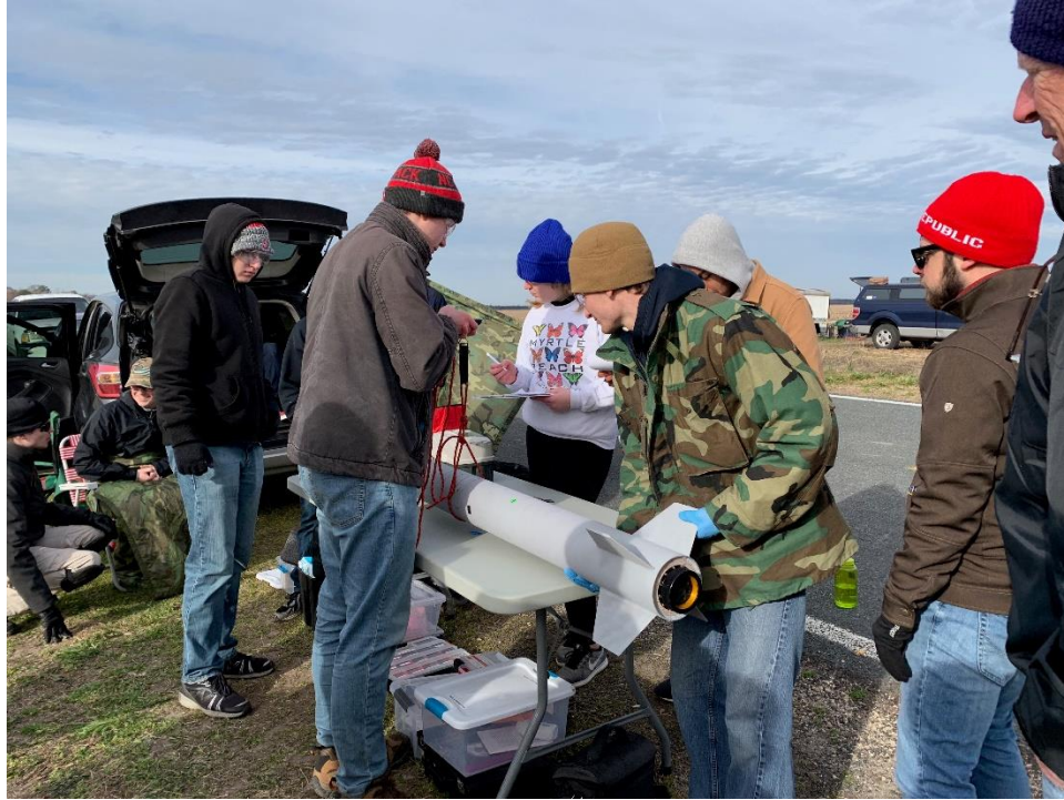
Figure 10-5 Measuring the CG of the fully assembled launch vehicle
