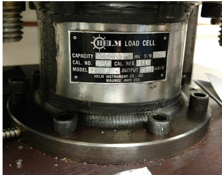
Figure 3-29: Helm Load Cell Used during Testing
