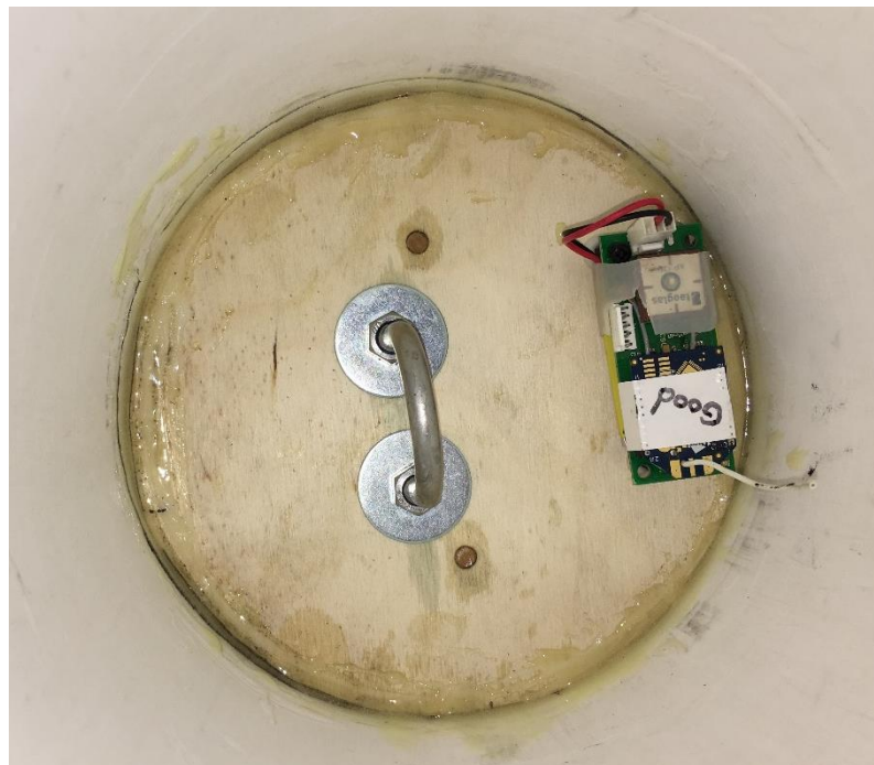
Figure 3-6: Nosecone Bulkhead with U-Bolt and GPS Transmitter
