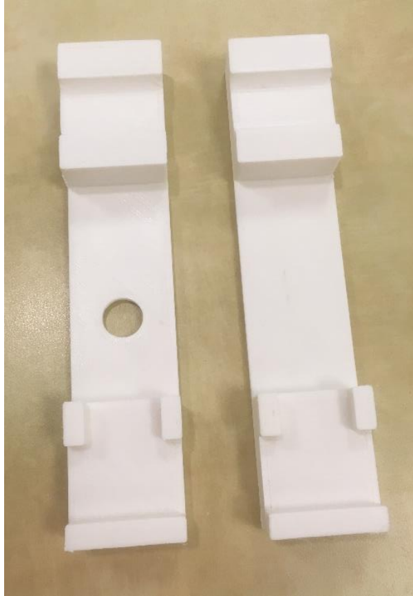
Figure 7-15: Shortened body split into two parts to increase print quality
