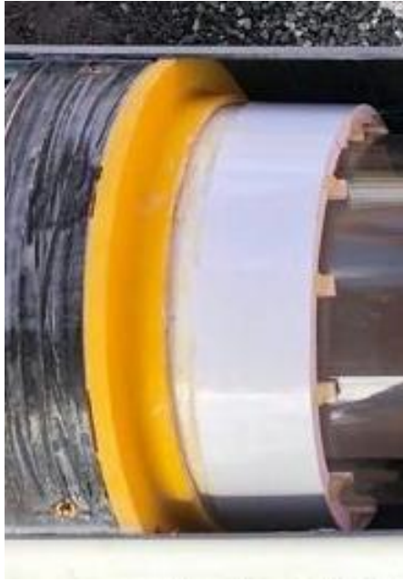
Figure 7-1: Forward Bearing with Sta-Lube Grease for Lubrication
