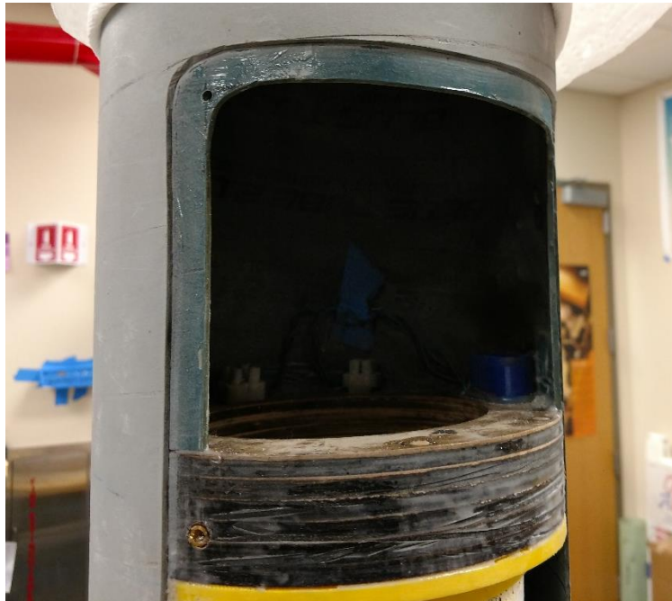
Figure 3-16: Forward Payload Centering Ring and Hatch Coupler
