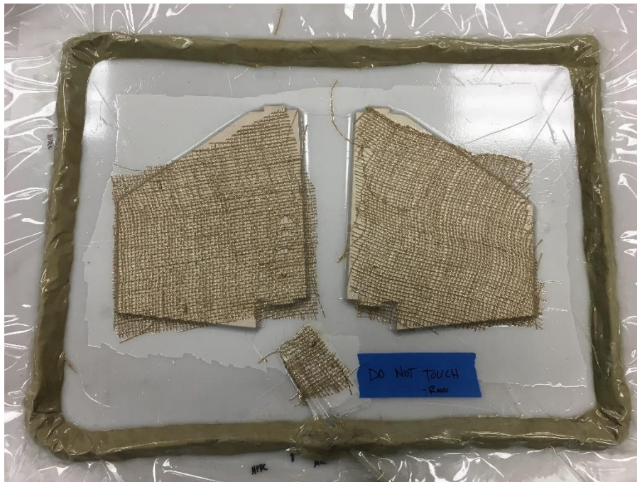
Figure 3-26: Fin Curing Process
