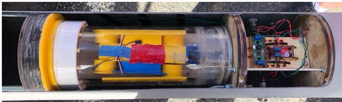
Figure 6-2: Assembled Payload and Avionics Bays Prior to Hatch Installation
