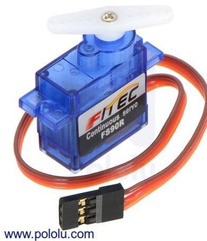
Figure 7-21: FEETECH FS90 Continuous Rotation Servo
