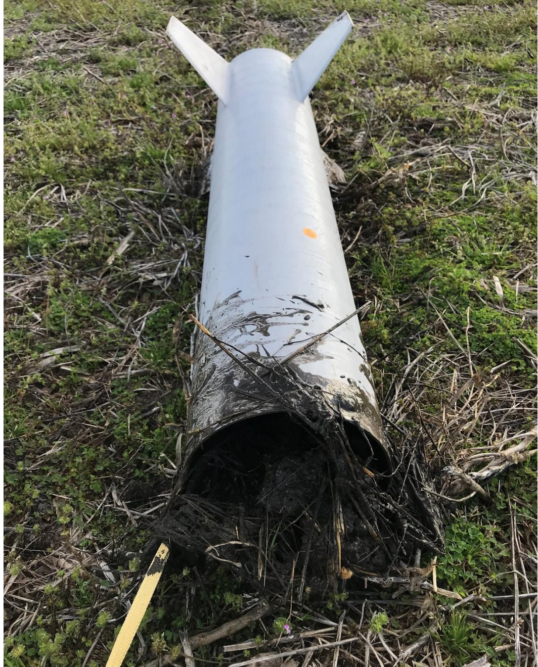
Figure 6-12: Fin Can Filled with Mud
