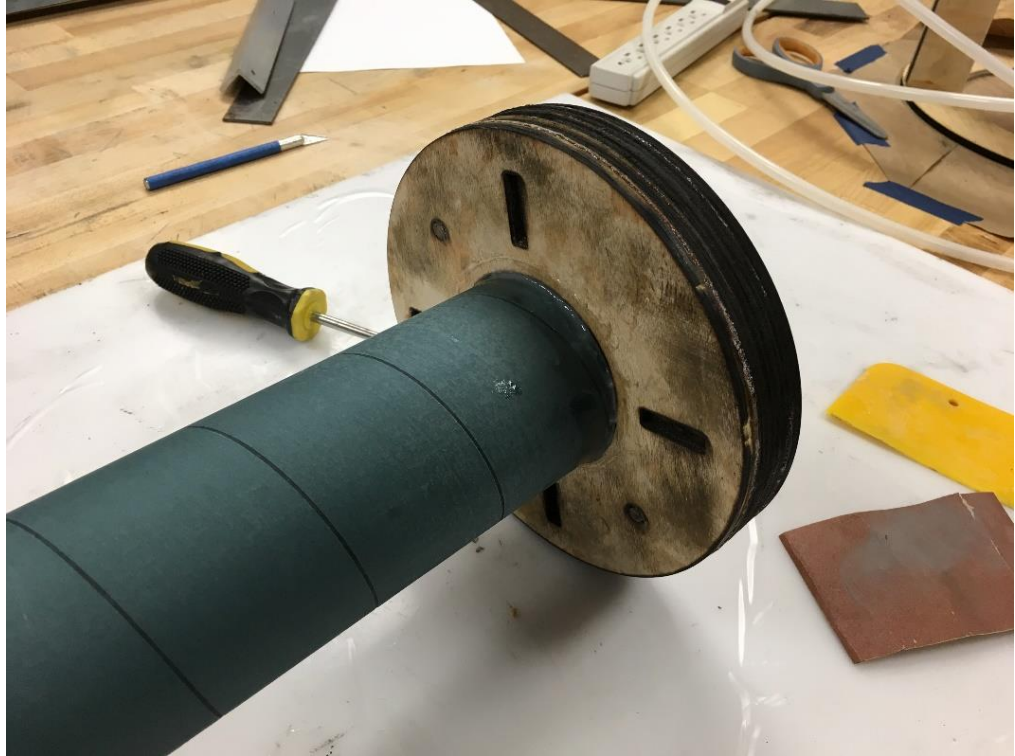
Figure 3-27: Motor Tube and Engine Block
