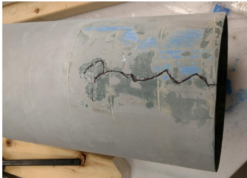
Figure 6-13: Bonded Midsection Zipper
