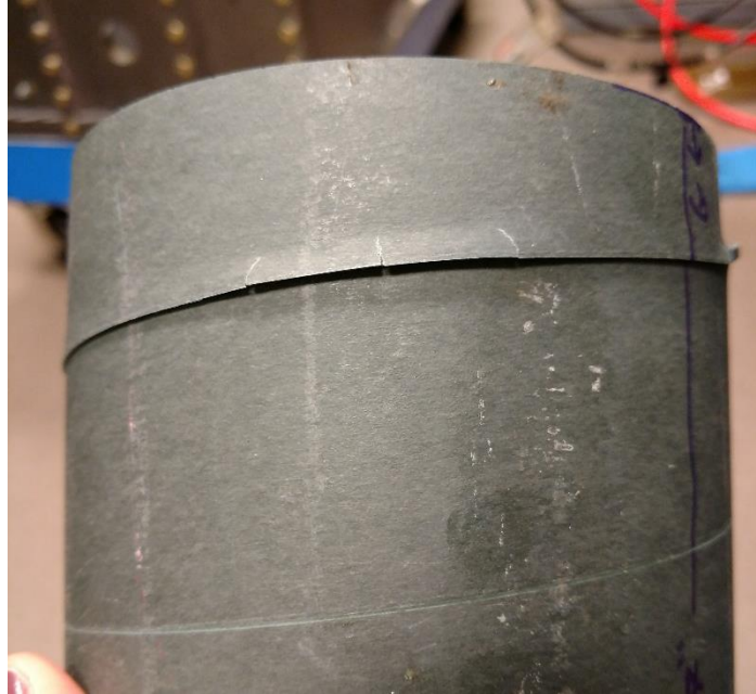
Figure 3-31: Buckled Blue Tube
