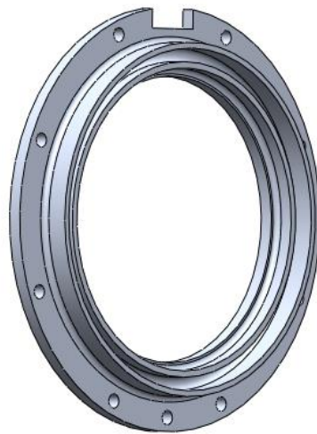
Figure 7-4: Model of the Aluminum Bearing Carrier
