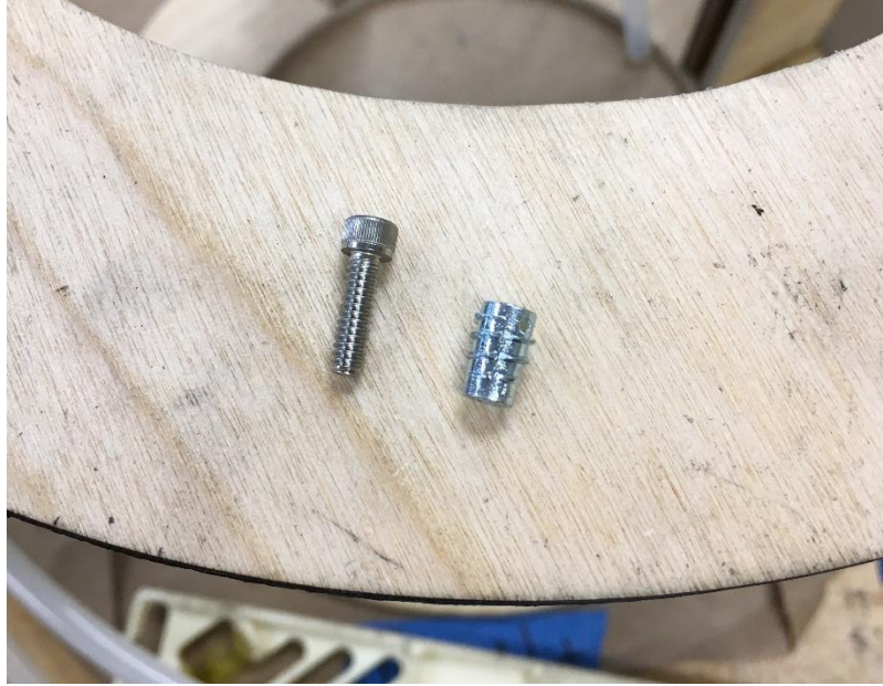
Figure 3-17: Nut Insert with #6-32 Bolt
