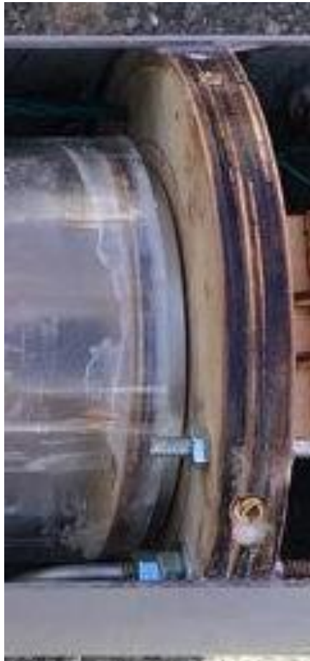
Figure 7-5: Aft Lazy Susan Bearing Installed on Full-Scale Launch Vehicle
