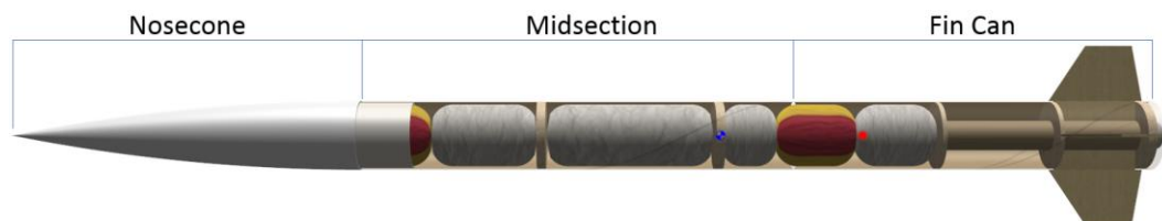
Figure 3-24: Subscale OpenRocket Model with Section Labels
