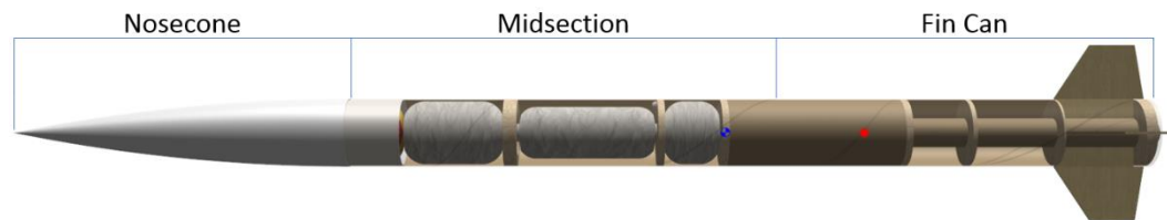
Figure 3-2: OpenRocket Model with Section Labels
