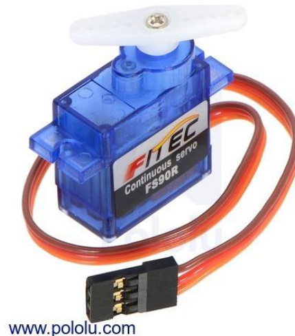
Figure 7-8: FEETECH FS90 Continuous Rotation Servo
