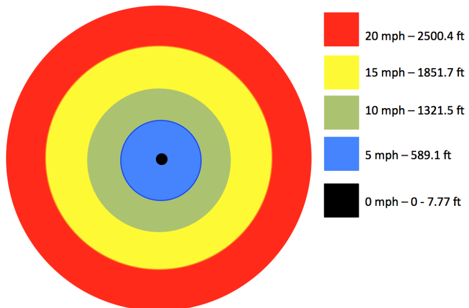
Figure 5-7: Radial View of Wind Drift Lateral Distances from Launch Pad
