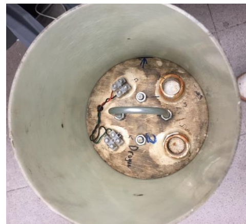
Figure 22: Aft. view of AV bay assembly with AV sled installed (left) and final aft. bulkhead installed (right)
