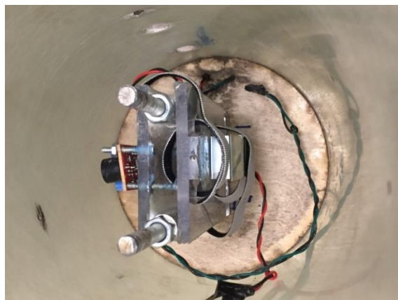
Figure 22: Aft. view of AV bay assembly with AV sled installed (left) and final aft. bulkhead installed (right)
