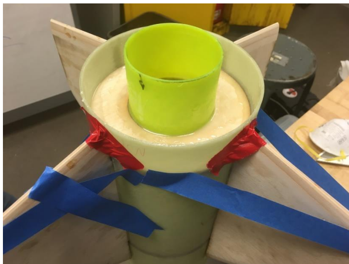
Figure 28: Aft. view of fin can, following final centering ring installation
