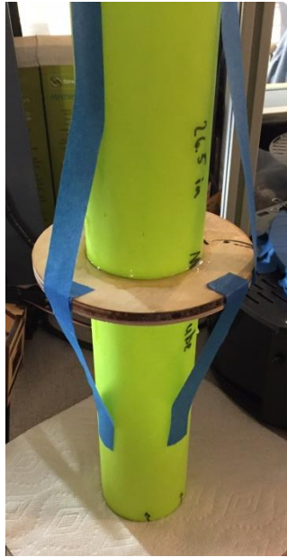
Figure 26: Motor tube and forward centering ring before and after (left. and right) being bonded to the fin can
