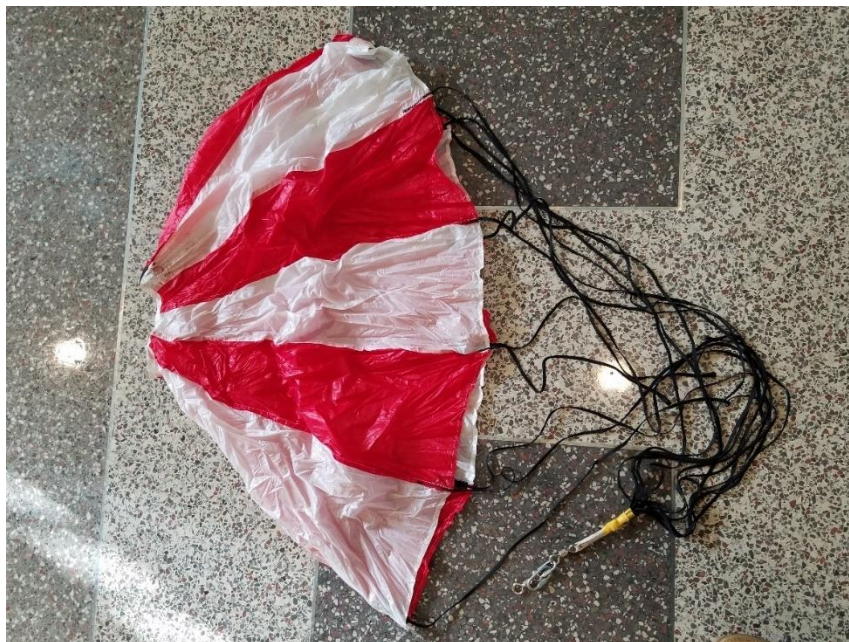
Figure 49: Payload 48in Diameter Parachute
