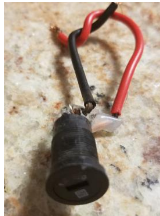
Figure 18: Rotary Switch for altimeter priming
