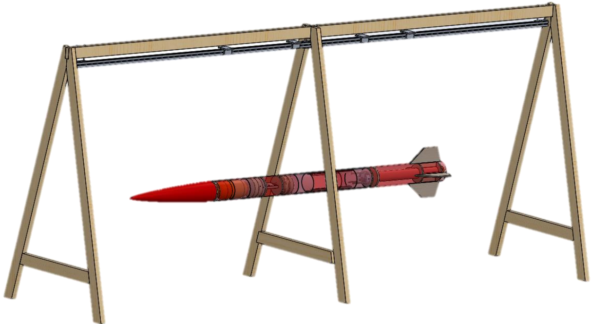
Figure 53:Deployment test rig with complete vehicle assembly (no supporting straps shown)
