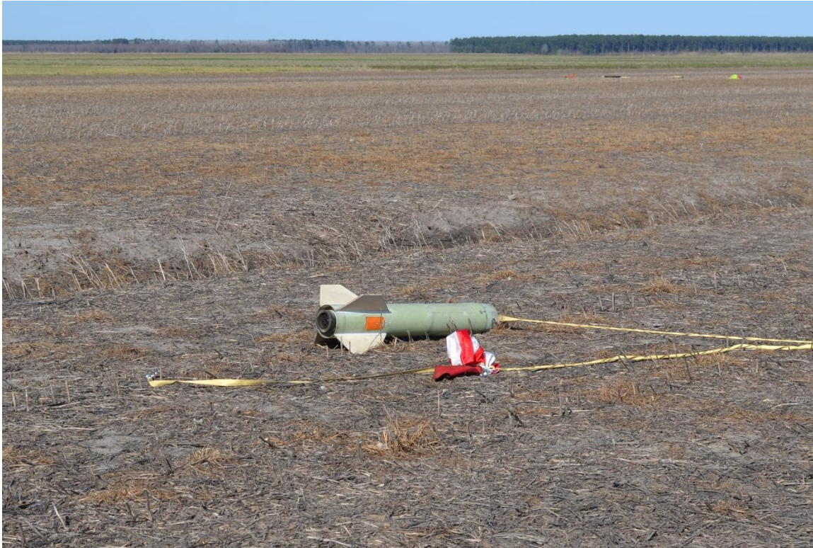
Figure 15 Photo of the Aft Airframe and Fin Section after a Successful Recovery
