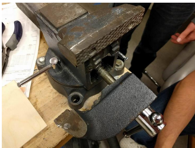
Figure 45 Sheared Vice Following Ratchet Test
