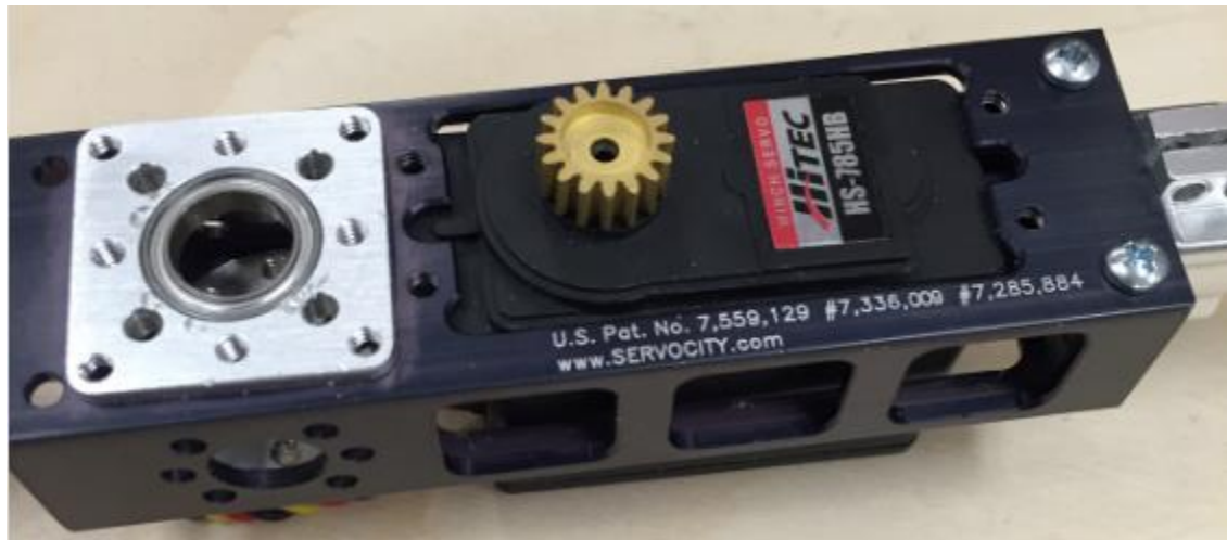
Figure 2 Stock Servo Fit in Motor Mount
