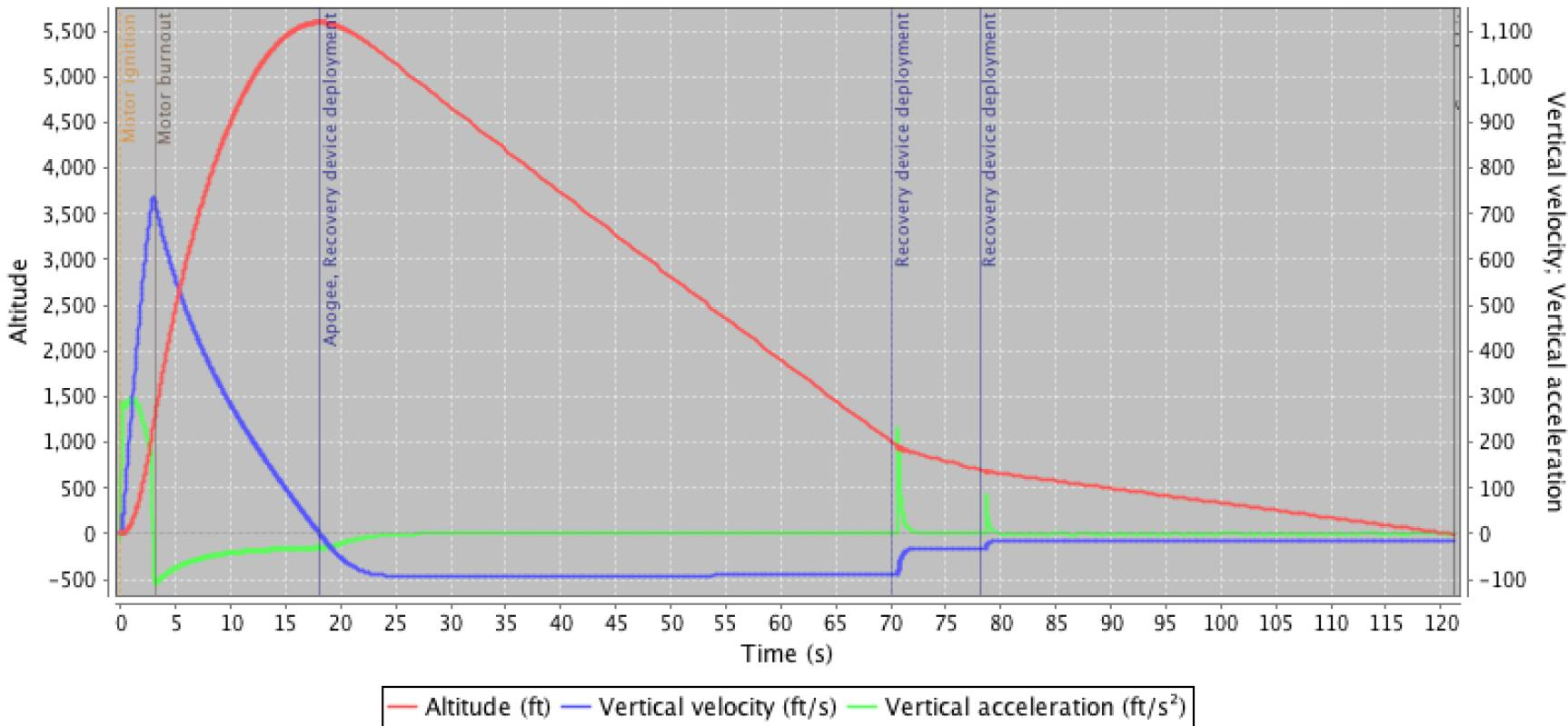
OpenRocket Simulation using AeroTech L1150
