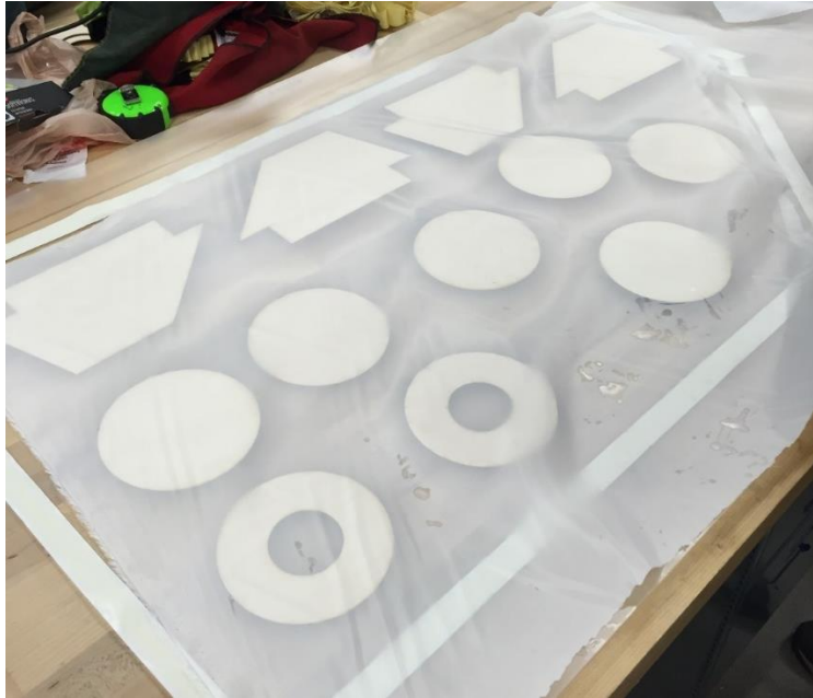
Figure 2 Fin and Bulkhead Layup
