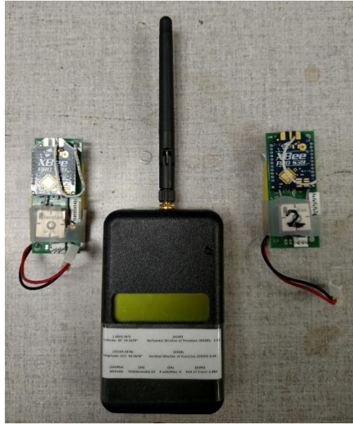
Figure 18 Forward and Rear Section GPS Transmitters and Receivers
