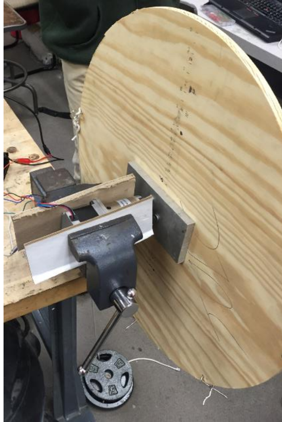
Figure 66: Launch Rail Stepper Motor and Pulley Apparatus
